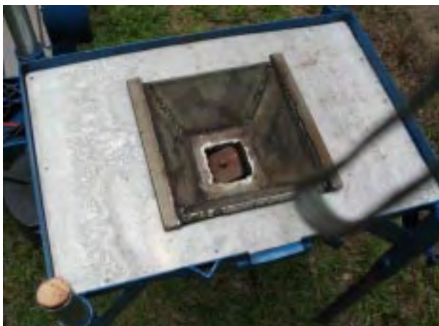
Figure 8: Forge pot & clinker breaker
