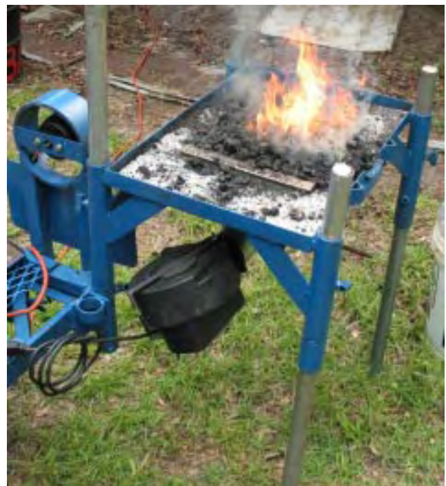
Figure 10: Forge with copier blower
