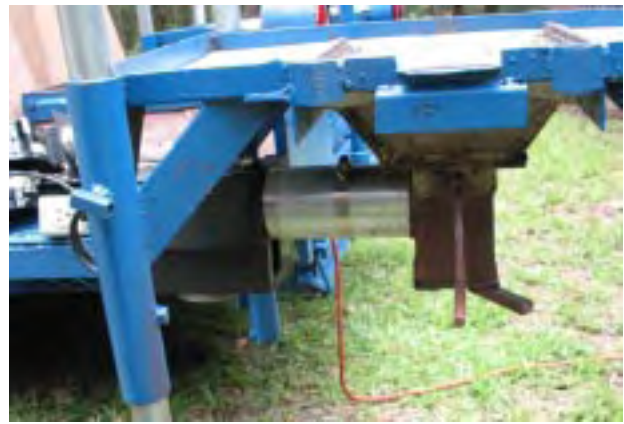
Figure 9: Tuyere and blower attachment
