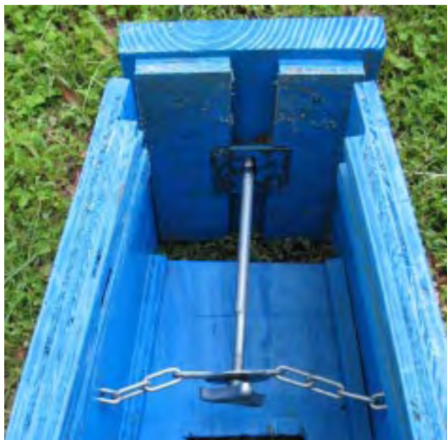
Figure 12: Anvil stand internal view
