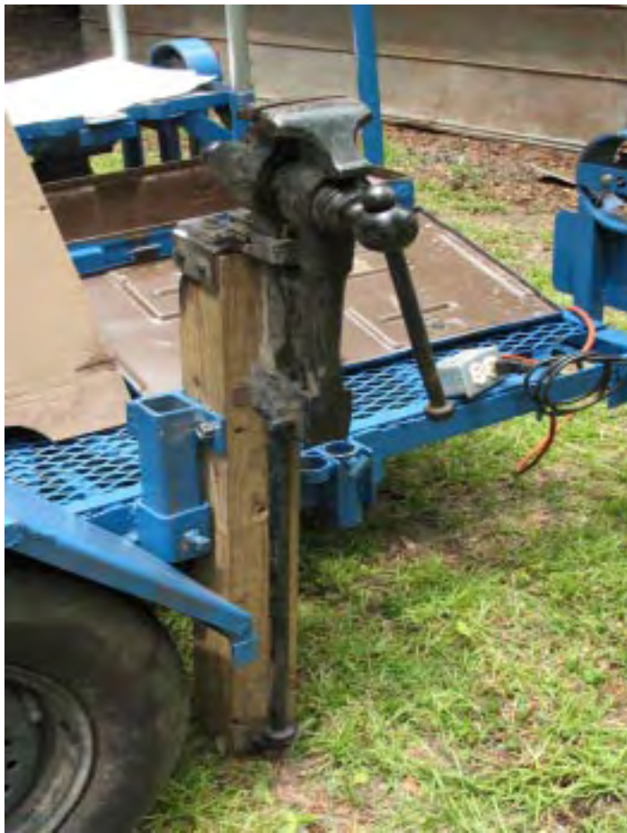
Figure 5: Post vise mount system
